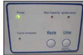
The burn cycles are controlled by a circuit board. A display panel signals when the burn cycles are completed, if fuel is out, or if there has been too many users in a too short time period, etc.
