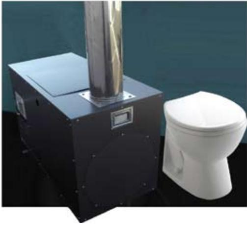
The WC Series consists of a few different WC models: WC5, WC32, and WC48. These systems are ideal in any remote application where a conventional toilet is too expensive or difficult to install. Since the WC units incinerate the black water, there is no need for pumping out any tanks or connect to a septic or sewage system. The WC systems operate along with one or several low flush toilets; grey water from sinks or showers can also be tied into to the system.
